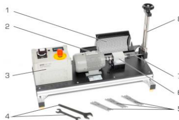
Fig. 2. GUNT WP 140 machine used to perform the different fatigue tests 1: Protective cover, 2: drive motor, 3: control center, 4: tools, 5: test pieces, 6: support, 7: test piece, 8: device to apply the load by rotating the black wheel on top.
