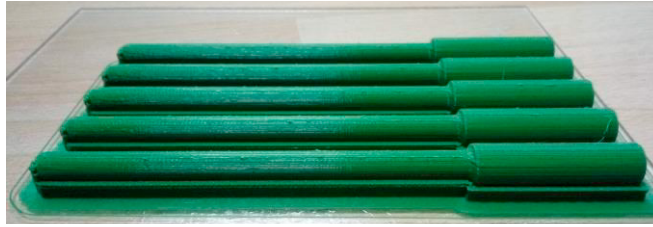
Fig. 3. Printing tray with 5 test pieces printed with the same parameters.
