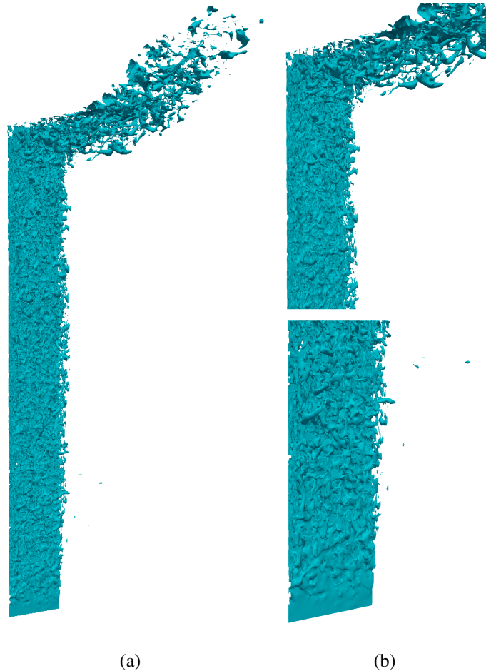
Figure 4: Instantaneous coherent structures for Q = 0.3 (a) whole cavity (b) details of the top and bottom of the cavity.
