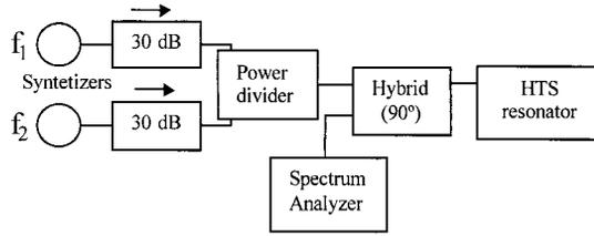
Fig. 5. Block diagram of the one port measurement setup.
