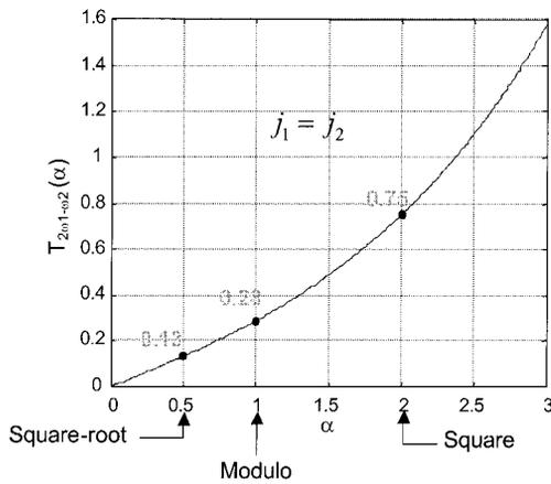
**Fig. 3.** Dependence of  $T_{2\omega_1-\omega_2}$  on the order of the nonlinearity  $\alpha$  for balanced current amplitudes. In this case, the amplitude of the electric field at the surface of the HTS at the intermodulation frequency will be proportional to  $T_{2\omega_1-\omega_2}(\alpha)j_1^{\alpha+1}$
