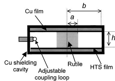
Fig. 4. Dielectric resonator structure used for IMD characterization of HTS films.
