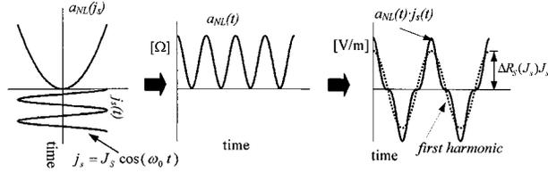
**Fig. 1.** Comparison between  $a_{\text{NL}}(t)j_s(t)$  in time domain (solid line in rightmost graph) and the deviation of the surface resistance from its small-signal value ( $\Delta R_s$  proportional to the amplitude of the sinusoid drawn with dotted line in the rightmost graph).
