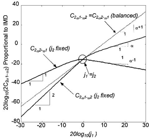
**Fig. 2.** Dependence of the electric field at the intermodulation frequencies ( $2C_{2\omega_1-\omega_2}$  and  $2C_{2\omega_2-\omega_1}$ ) on the amplitude of the surface current  $j_1$ .
