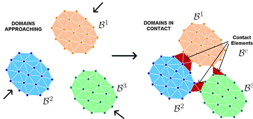
Figure 1: Geometric contact detection in the PFEM.
