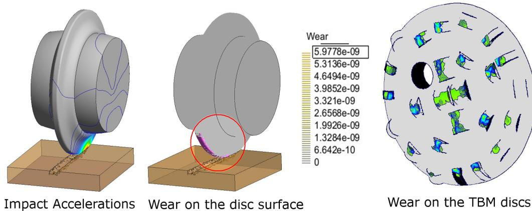
Figure 4: Wear on a TBM hear and on one of its cutting discs.
