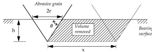
Figure 2: A simplified abrasive wear model showing how a cone removes material from a surface
