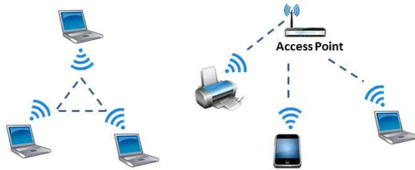
Figure 1.9 Independent and infrastructure basic service sets (BSSs).
