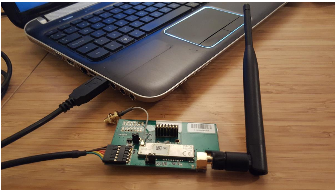
Figure 3-7. EVB TD1204 connected to the PC with antenna. [own source]
