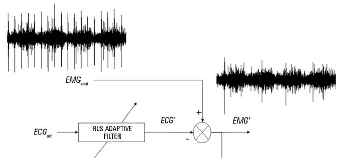
**Figure 1** - Scheme of the adaptive filter process using RLS algorithm. Where  $EMG_{real}$  is the recorded EMG signal that was bandpass filtered,  $ECG_{art}$  is an artificial ECG signal obtained from  $EMG_{real}$ ,  $ECG'$  is the ECG obtained from adaptive filter and  $EMG'$  is the EMG with a reduced cardiac interference.  $EMG_{real}$  - real electromyogram;  $ECG_{art}$  - artificial electrocardiogram; ECG - electrocardiogram.
