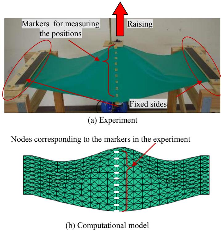
Figure 5: Large deformation of the suspended membrane
