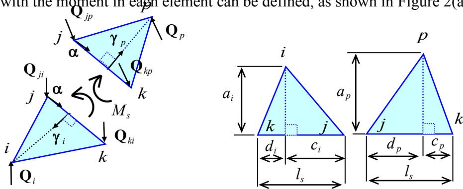
(a) End shear forces balanced with the end moment
