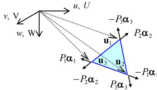
Figure 1: Element end forces in the plane
