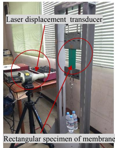
Figure 4: Test for measuring material constants
