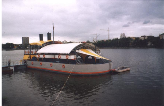
Figure 11: A tent structure as an awning over a boat deck on the Iset river
