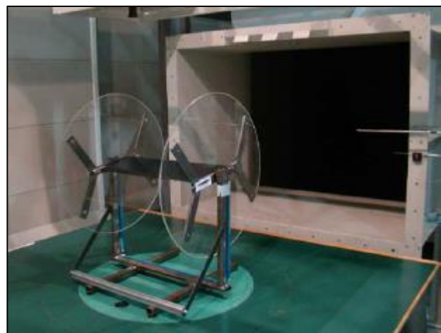
Figure 8 – Elasto-flexible 2D model mounted in wind tunnel test section
