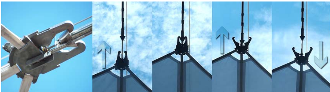
Figure 2: autonomous mechanical clamping system
