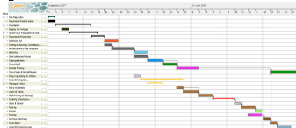
Figure 7 - Overview of the entire Construction Process
