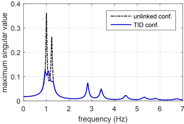
Fig. 4. Interstory-drifts frequency response for the TID configuration.
