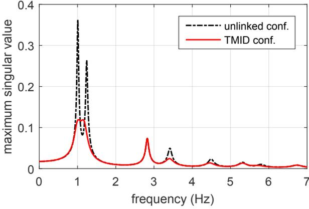
Fig. 2. Interstory-drifts frequency response for the TMID configuration.
