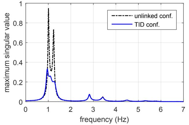
Fig. 5. Interbuilding-approaches frequency response for the TID configuration.
