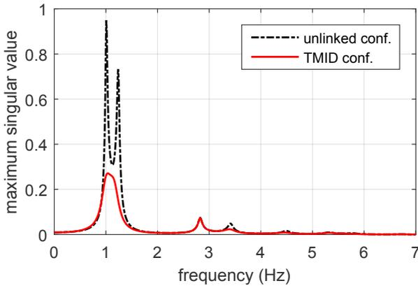
Fig. 3. Interbuilding-approaches frequency response for the TMID configuration.
