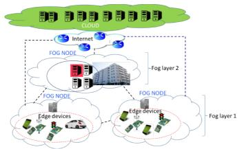
Figure 1. Fog-to-cloud architecture (F2C)
