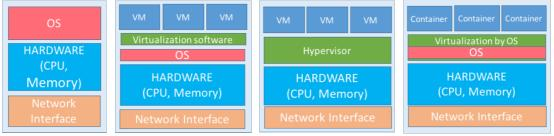
a) Basic edge device b) Virtualized type 1 c) Virtualized type 2 d) Virtualization by OS
