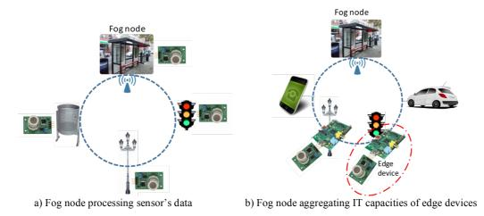
Figure 2. Illustrative example for the two categories of fog nodes
