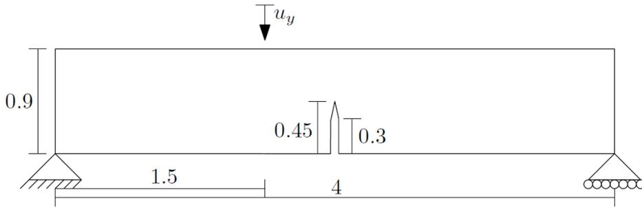
**Figure 4:** Notched beam on two supports with a punctual displacement imposed on the top.
