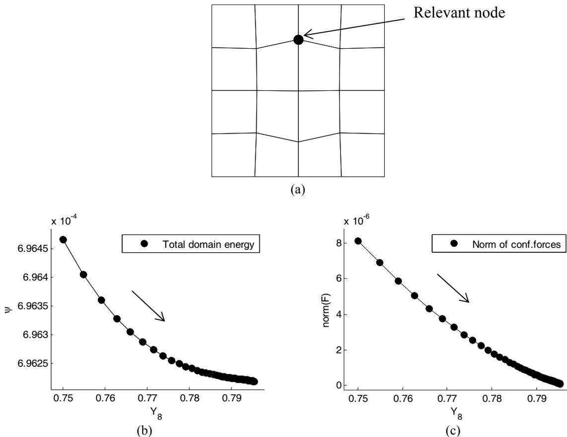
**Figure 3:** (a) Optimal mesh configuration. (b) Total mesh energy with respect to relevant node vertical position, and (c) norm of configurational forces with respect to relevant node vertical position.
