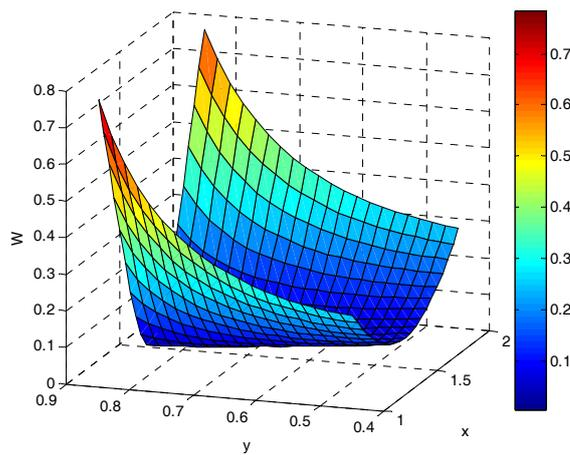
**Figure 6:** Total domain energy as a function of the central node position.
