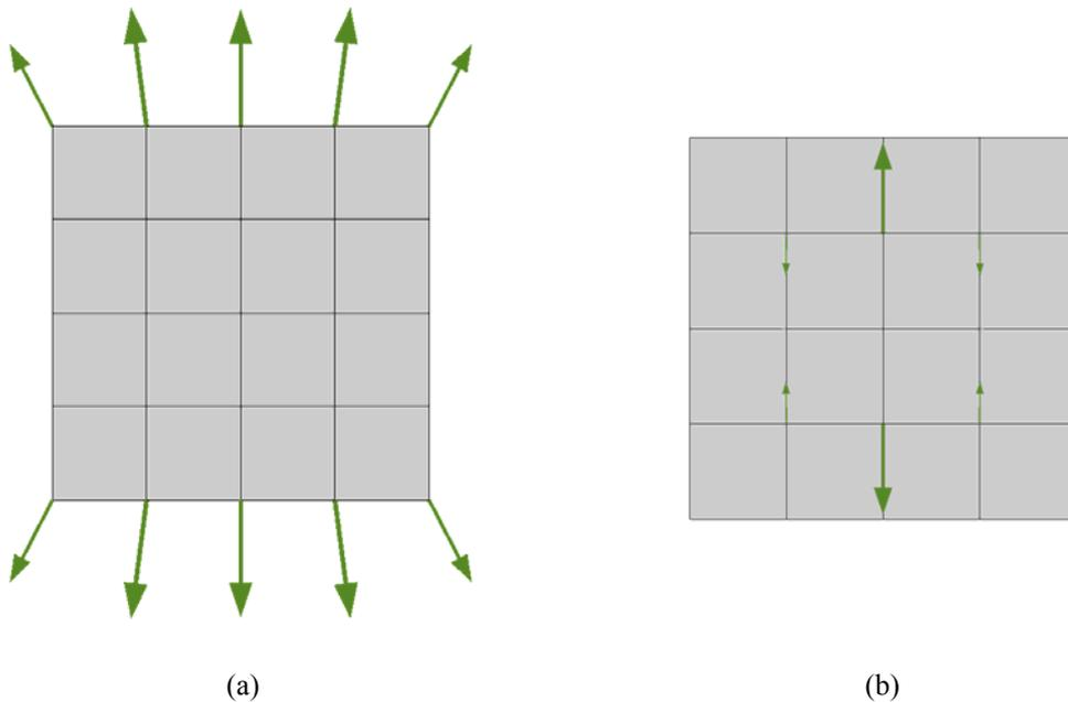
**Figure 2:** (a) Configurational forces (with minus sign) on all nodes of the mesh, at the scale dictated by larger forces on the boundary nodes, (b) same only for internal nodes, at a larger scale in which forces on those nodes would be represented.
