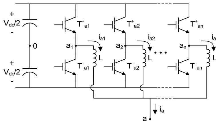
Fig. 1: A single phase of a VSI integrated by  $n$  legs connected in parallel
