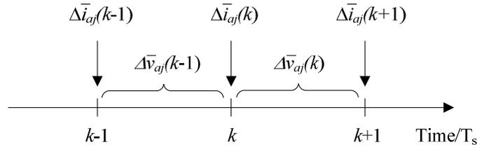
Fig. 3: Time sequence of the sampling process for current balancing
