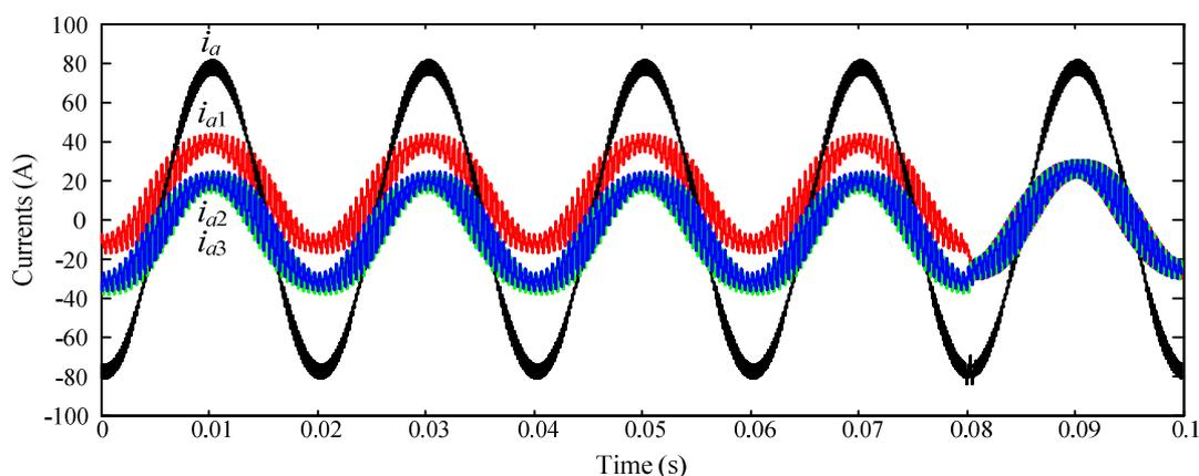
Fig. 6: Simulation results assuming different voltage drops on the power devices. The balancing control is activated at the time 80 ms
