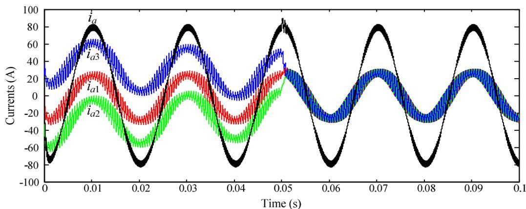
Fig. 5: Simulation results for an initial current imbalance. The balancing control is activated at the time 50 ms
