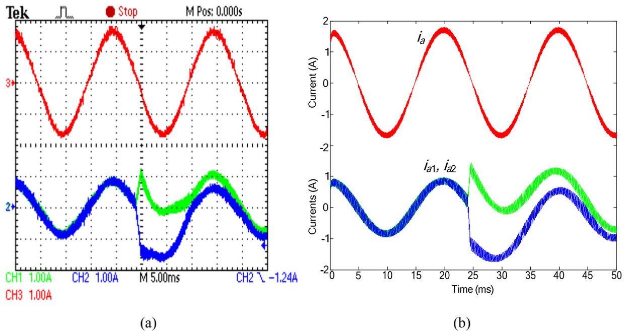
Fig. 7: Two parallel legs operating without the balance compensator: (a) experimental and (b) simulation results
