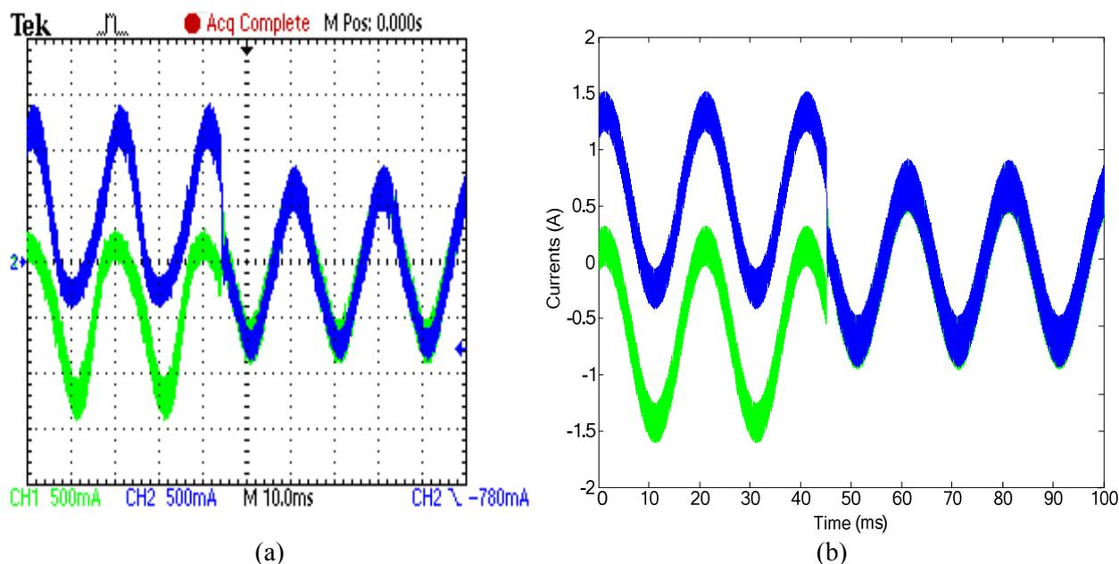
Fig. 9: Current imbalance produced by a small dc voltage difference between the legs and activation of the compensator: (a) experimental and (b) simulation results
