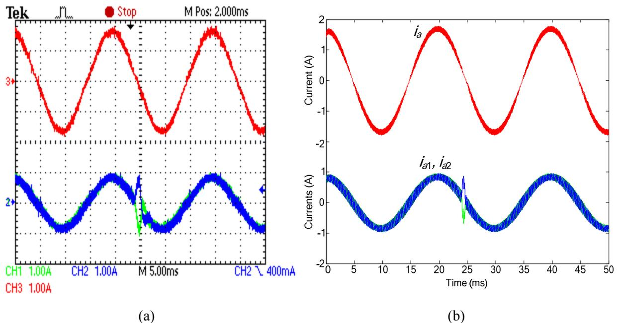
Fig. 8: Two parallel legs operating with the balance compensator activated: (a) experimental and (b) simulation results
