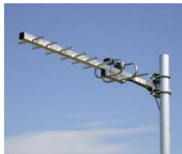
**Figura 3.5.** Antena Yagi
