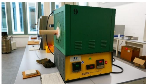
Figura 3.26 Forn tubular Hobersal mod. ST-18.
