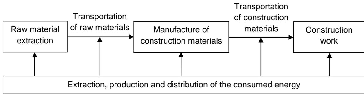
**Figure 2.** Cradle-to-gate stages in construction considered by the model.
