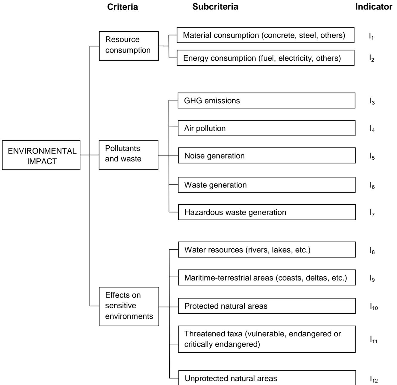
**Figure 3.** Impact tree with the environmental impacts caused by construction work.
