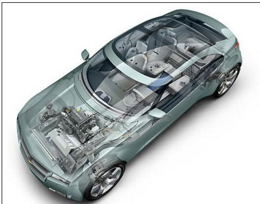
Figura A.7. Powertrain Chevrolet Volt (Dash Z Racing, 2008)
