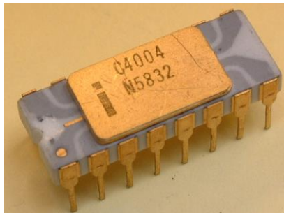
Figure 1.1.3. i4004. First microprocessor of the history.
