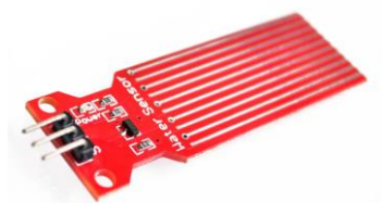
Figure 3.2.8. DIY T1592 water level sensor.
