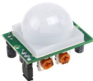
Figure 3.2.6. PIR movement sensor.
