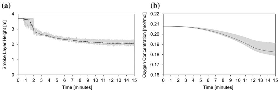
**Figure 3. (a) Evolution of the smoke layer height and (b) the oxygen concentration inside the nacelle. Black lines represent average values calculated throughout the nacelle (divided in 10 meshes). Grey shadowed areas comprise the region between maximum and minimum values.**
