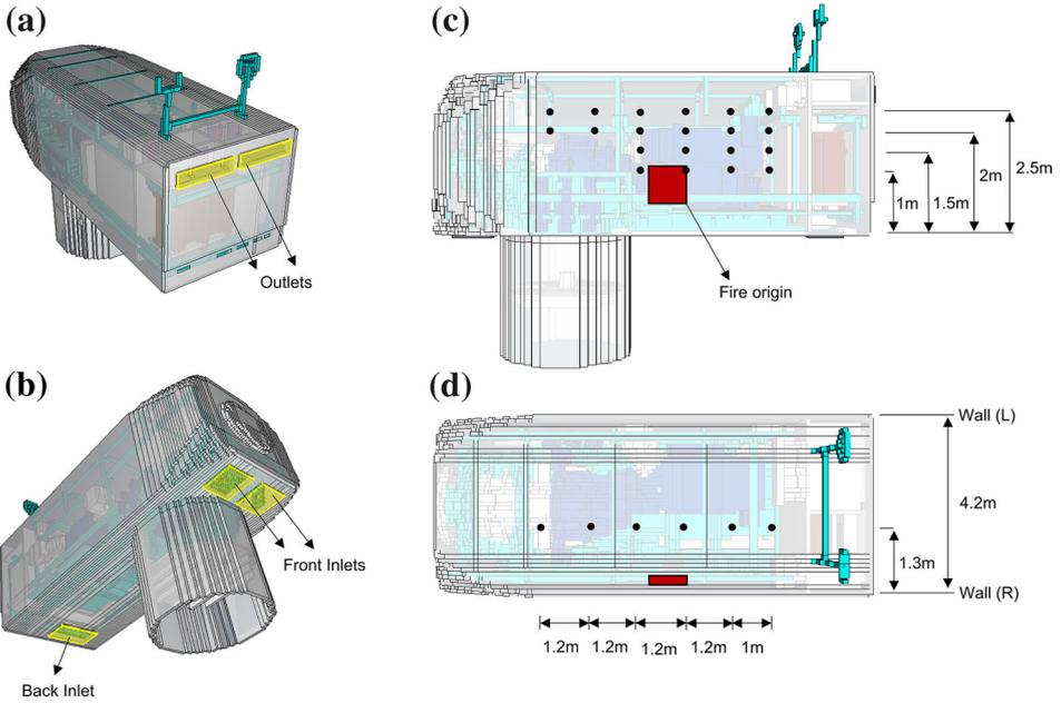
**Figure 2. Distribution of the (a) outlet and (b) inlet vents that compose the natural ventilation system; (c) height and (d) plan view with details on the location of measurement points (black dots) and fire origin (red surface). (L) left, (R) right.**
