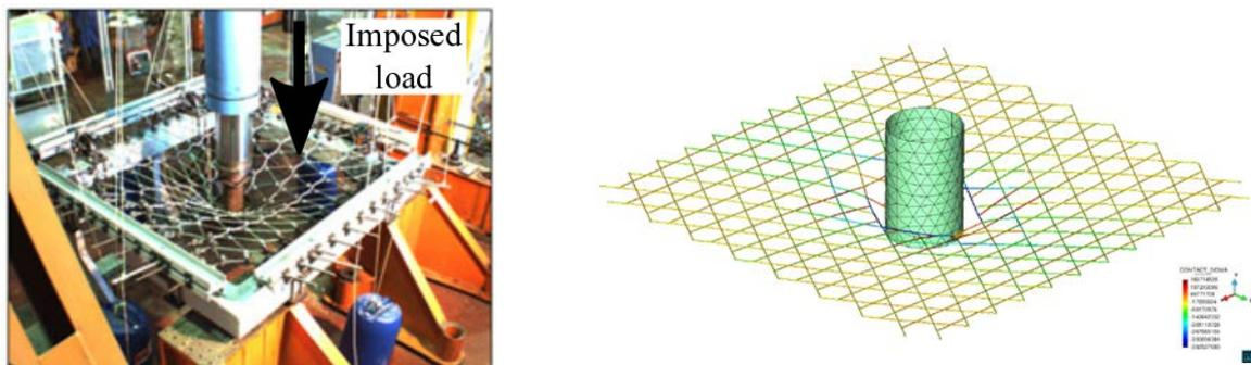
Fig. 3 Laboratory [1] (left) and numerical model (right) of the second validation test.
