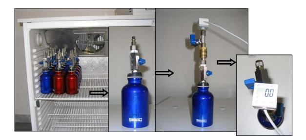
Figure 3.4. Incubation and biogas measurement during anaerobic batch tests (Ferrer et al., 2004b)
