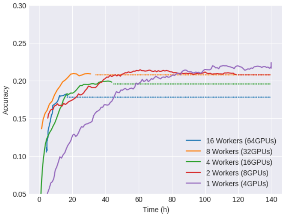
Figure 3.8: Test accuracy evolution until convergence in different asynchronous distributed configurations.
