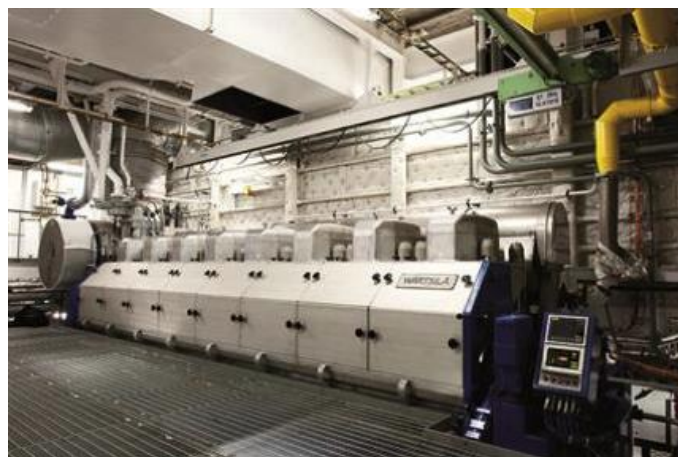
Figure 4.6: Wärtsilä 8L50DF engine on board Viking Grace (Source: Wärtsilä n.d.-b).
