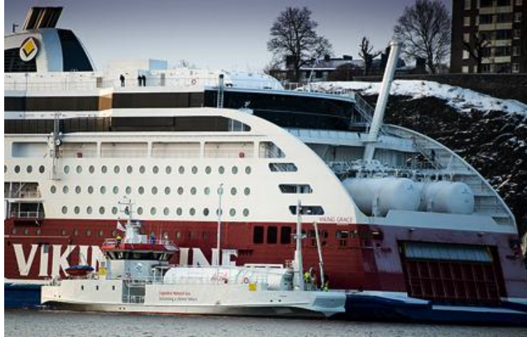
Figure 4.5: Viking Grace undergoing LNG bunkering operations at Port of Stockholm (Source: Faber et al., 2015).
