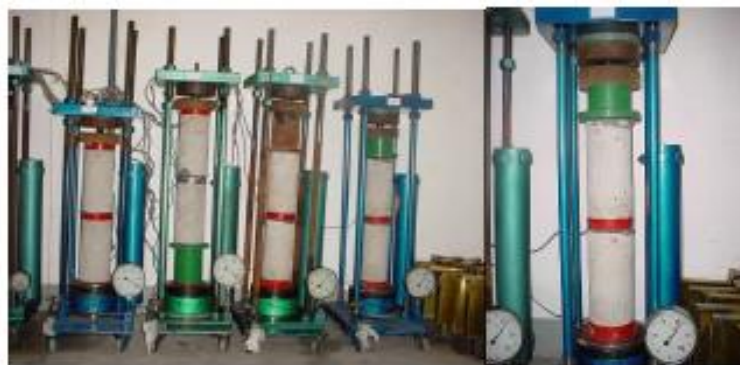
Figure 7. Creep test in the LTE (De La Cruz, 2006)
