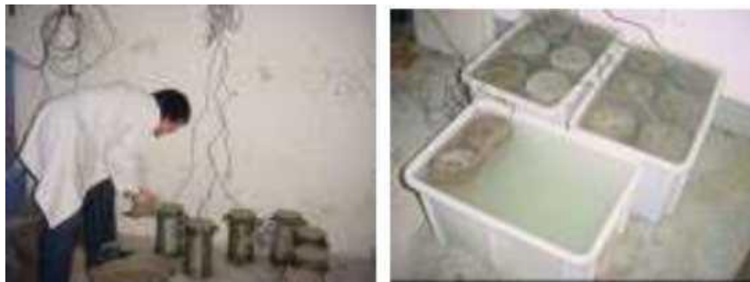
Figure 2. Procedure shrinkage and creep test on specimens of SCC-MS (De La Cruz, 2006)
