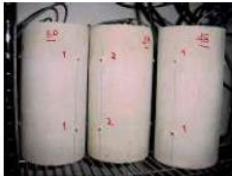
Figure 3. Test tubes with strain measurement points on the surface and attached comparator DEMEC N°8865 lengths. (De La Cruz, 2006)
