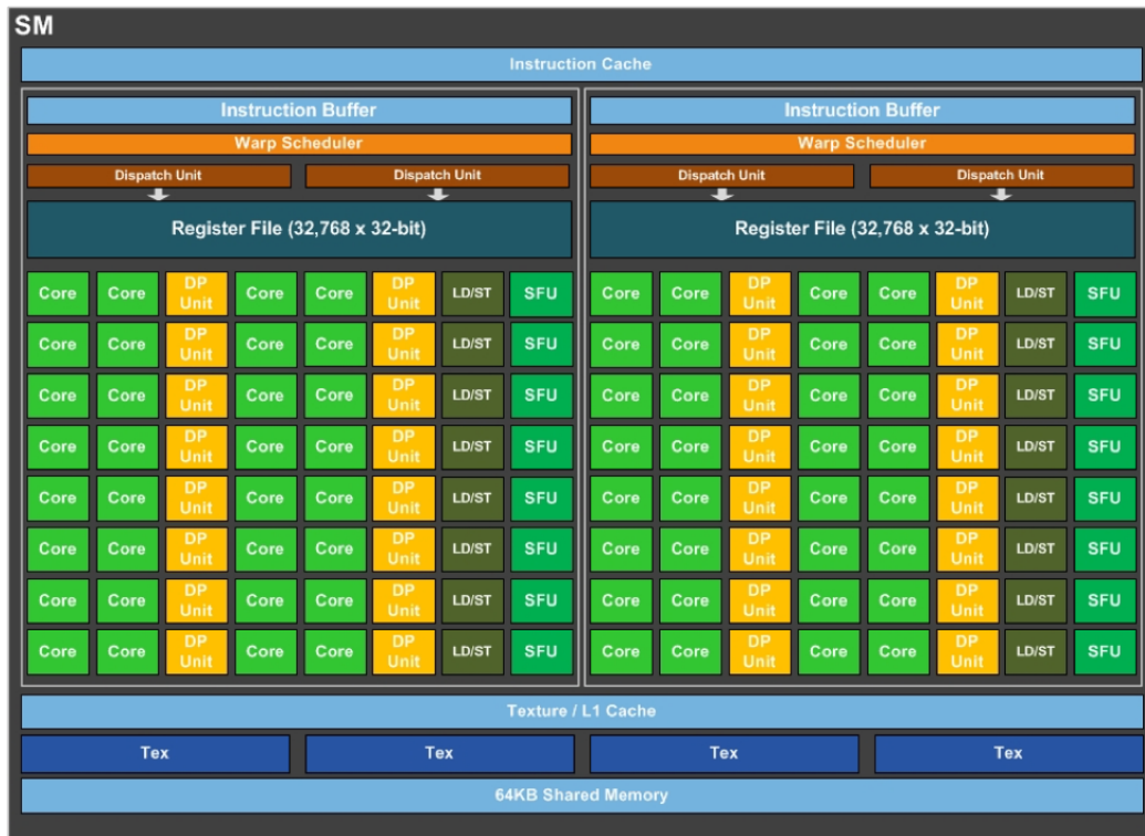
Figure 2.2: SM in Pascal architecture [2]
