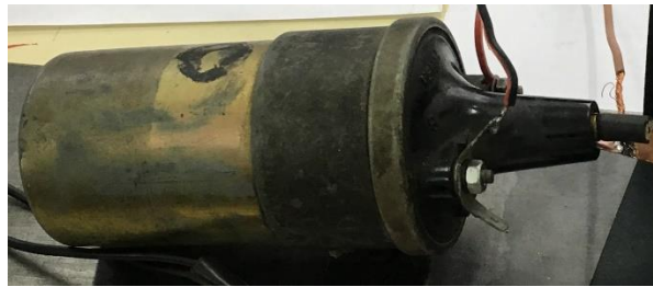
Figure 42. Ignition coil used in the first experiment.
