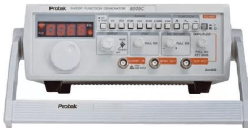
Figure 41. PROTEK sweep function generator 9205C used in the experiment #3.
