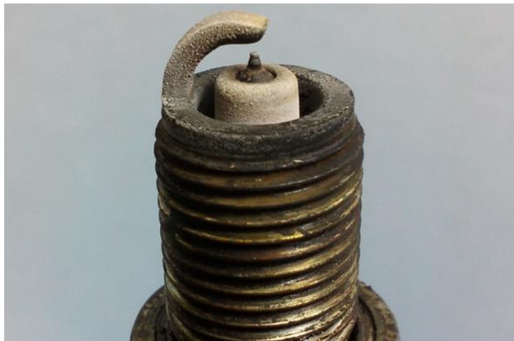
Figure 16. Erosion of a spark ignition system electrode.
