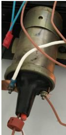
Figure 43. Ignition coil used in the 2nd and 3rd experiments.
