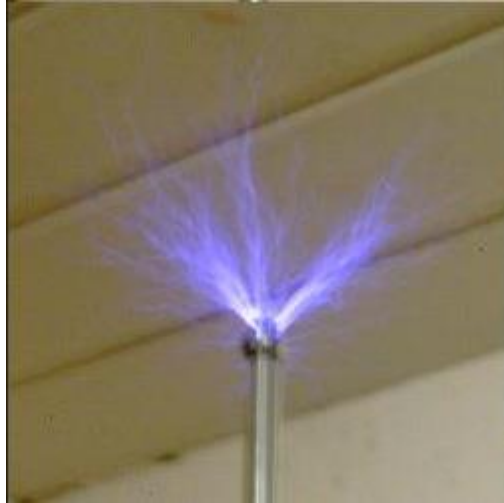
Figure 15. Streamers of the Streamer Corona.
