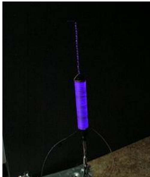
Figure 12. Glow light caused by corona discharge surrounding a high voltage coil.
