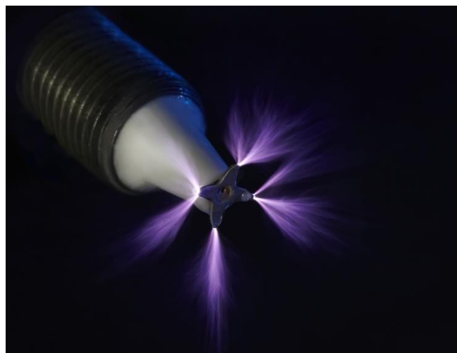
Figure 20. Electrode tips of the Federal-Mogul ACIS igniter.
