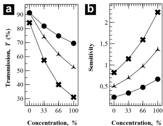
Fig. 8. (a) Evolution of the peak's amplitude when exposed to 0%, 33%, 66% and 100% of gas concentration in for the number of periodicities  $N$  (●) 5, (×) 7, and (▲) 9. In all cases  $l = 20 \mu\text{m}$ . (b) Sensitivity in the three cases.
