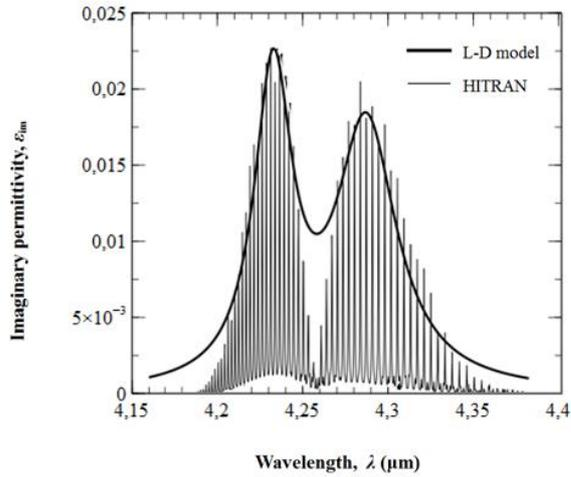
Fig. 2. Absorption lines for  $\text{CO}_2$  and the Lorentz-Drude approximation used in this paper which consists on modeling the gas absorption as the envelope (dark) of his absorption lines (grey).
