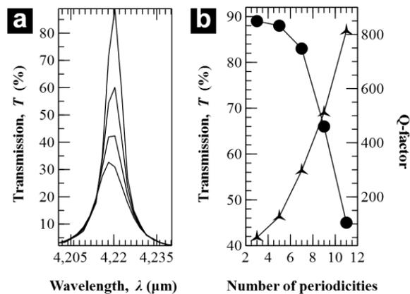
Fig. 6. Detail of the peak amplitude change with gas concentration. The MPS device has 9 modulation periods and a tail section of length  $l = 20 \mu\text{m}$ . In (a) the peak amplitude clearly decreases for  $\text{CO}_2$  concentration of 0%, 33%, 66%, and 100%. In (b) the peak's amplitude ( $\bullet$ ) and Q-factor ( $\blacktriangle$ ) dependence to the number of periods is plotted.
