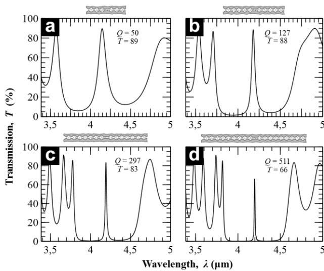
Fig. 5. Evolution of the amplitude and the Q-factor with respect of the number of periods: (a) 3 periods, (b) 5 periods, (c) 7 periods, and (d) 9 periods. The actual structures are depicted above the graphs for each case.
