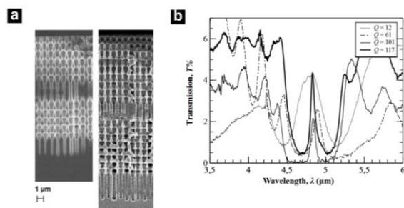
Fig. 7. (a) Scanning electron microscope (SEM) image of two photonic crystals with  $N = 5$  and  $8$ , respectively. The tail has been lengthened until  $6.5 \mu\text{m}$  in both cases. (b) Transmission spectra of the structures with and without tail:  $N = 5$  and  $L = 0 \mu\text{m}$  (dotted line),  $N = 5$  and  $L = 6.5 \mu\text{m}$  (dot-dashed line),  $N = 8$  and  $L = 0 \mu\text{m}$  (light-black line),  $N = 8$  and  $L = 6.5 \mu\text{m}$  (dark-black line).
