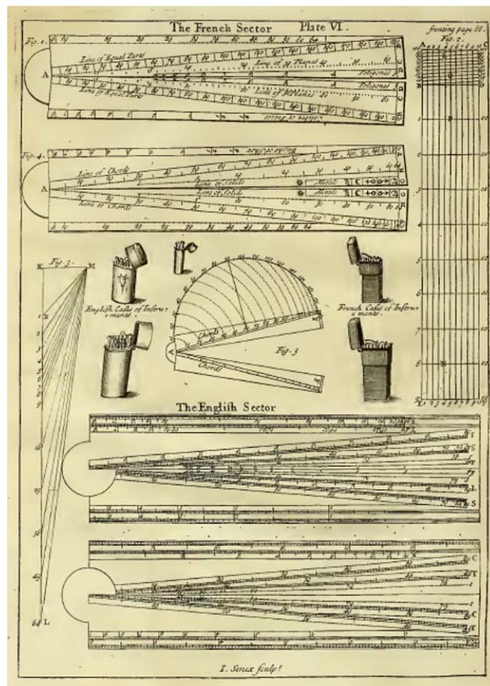
Figure 2. The French sector and the English sector, in Stone (1723), plate VI [digitized by the Internet Archive, 2012, with funding from Gordon Bell, available at <http://archive.org/details/constructionprin00bion>]
