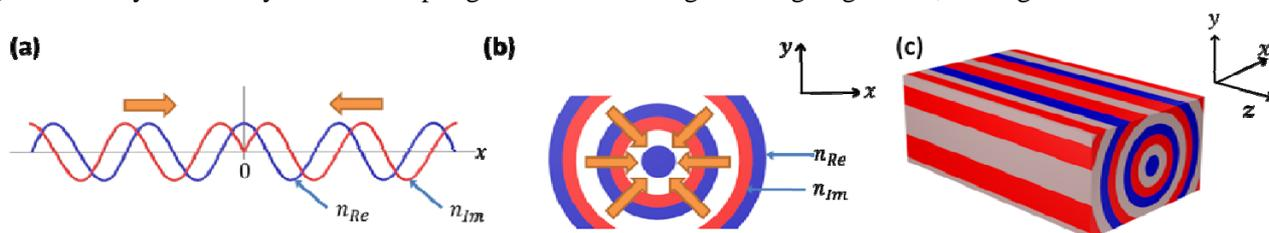
**Figure 1.** Local unidirectional coupling: (a) 1D complex optical potential, where  $n_{Re}$  is the real index modulation, and  $n_{Im}$  the gain/loss modulation. (b) 2D analogous axisymmetric configuration, (c) 3D coaxial index and gain/loss modulations, analogous for fields propagating along  $z$ . The arrows indicate the direction of the asymmetric mode coupling, at resonance.
