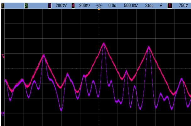
Fig. 9. FPGA generated envelopes: DACs outputs ( $E_s(n)$  in red, and  $E(n)$  in violet).
