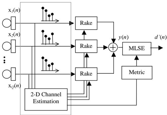
**Figure 1. Vectorial Rake Receiver.**
