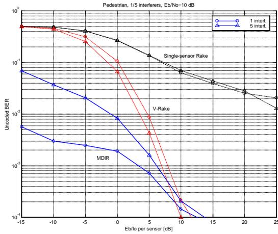
**Figure 3. Uplink results for the Pedestrian Channel Model.**
