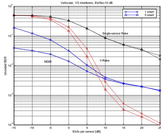
**Figure 4. Uplink results for the Vehicular Channel Model.**
