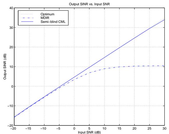
**Figure 8. Evolution of the SINR at the output of the beamformer as the users' power increases.**
