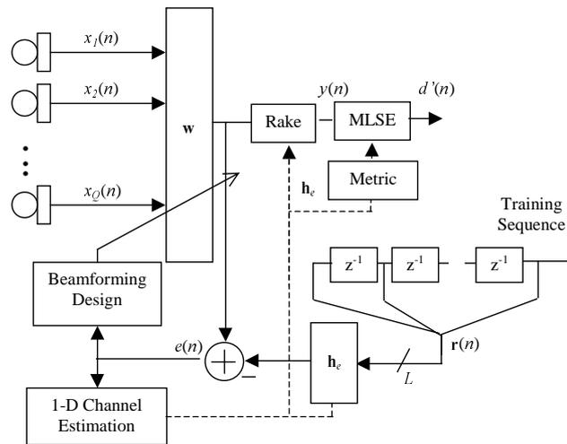
**Figure 2. Matched Desired Impulse Response Receiver.**
