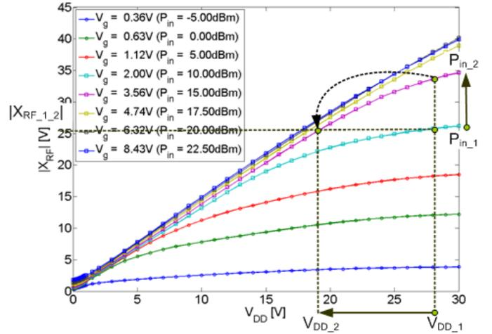
Fig. 3.  $V_{DD}-|x_{RF}|$  characteristics for a 15 W GaN HEMT PA.
