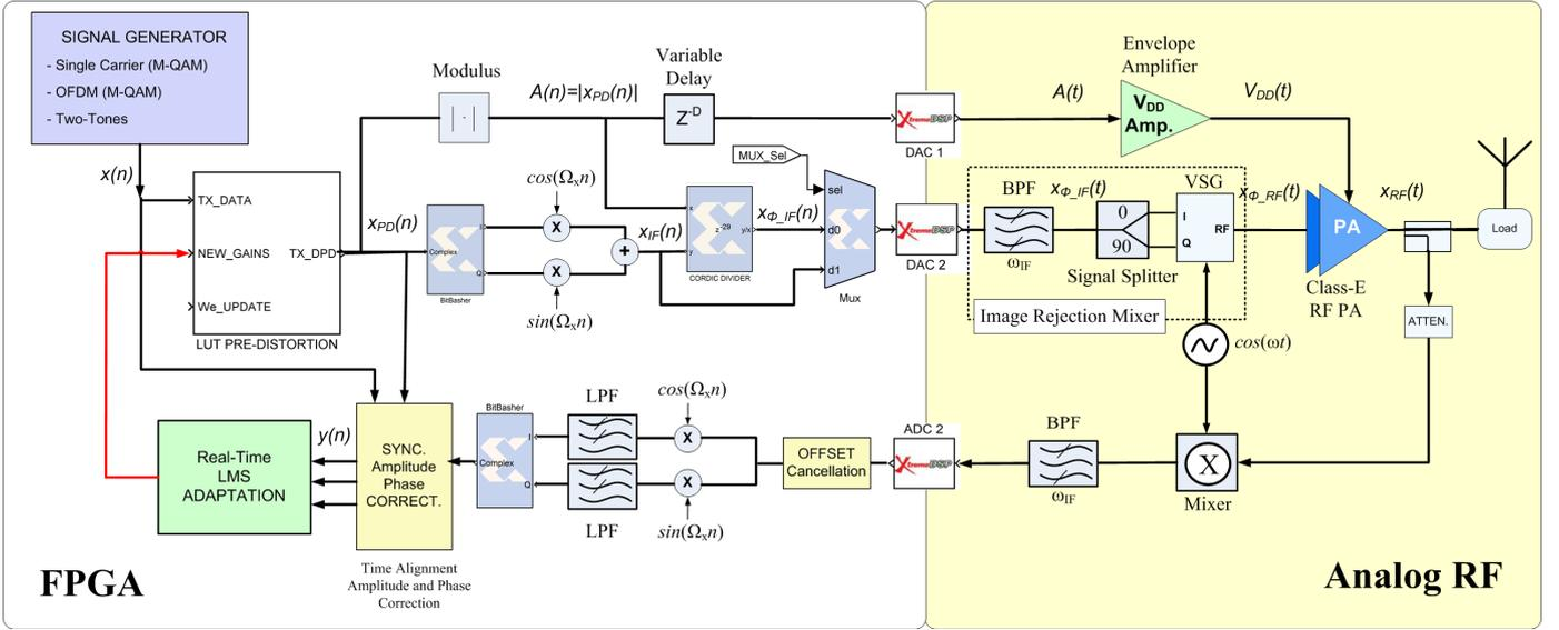
Fig. 1. Block diagram of a Polar Transmitter with real-time adaptive digital predistortion
