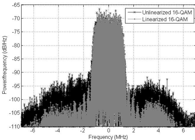
Fig. 6. 16-QAM output power spectra in the case of  $P_{in_2}$ .
