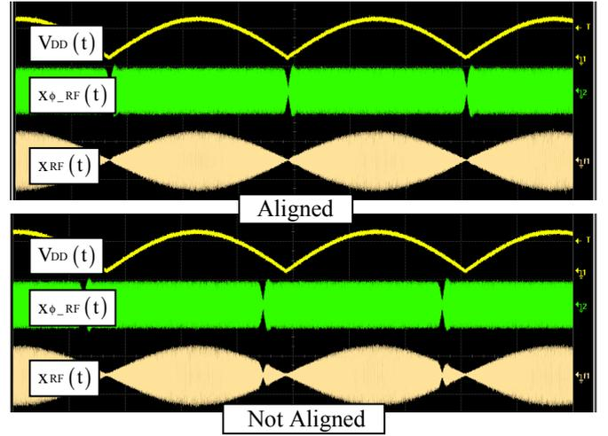
Fig. 2. Measured time-domain waveforms of a two-tone test.
