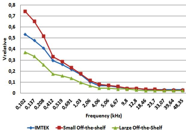
Fig. 3. Indoor solar panel responses to different frequencies.
