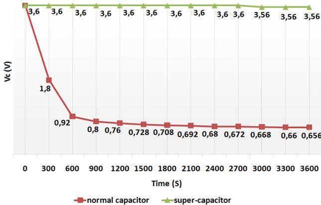
Fig. 4. Leakage test results for the electrolytic capacitor of  $470\mu F$  and super-capacitor of  $1F$ .
