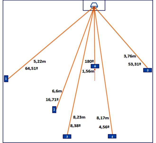
Fig. 6. Positions (distance and angles) tested with high probability of detecting wake-up frames.
