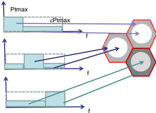
The thresholds of SINR are used to decide whether a UE has to be considered a cell edge UE or not. They are obtained by considering the SINR value for the worst case (assuming that all the eNB are using all the RBG simultaneously and with the same transmitted power). Threshold values are the same than in [4]. A better way to classify UEs is the one described in [4] according not only on their SINR but also on the EESIR and CQI parameters. This has not yet been introduced in the algorithms.
