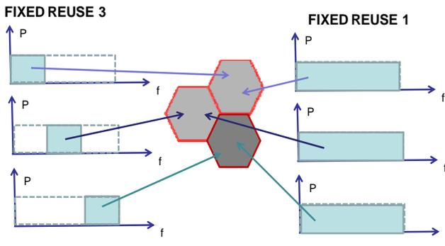
Reuse 1 is a good option for scenarios with low traffic while reuse 3 is better for high load scenarios. Reuse 1 in high load scenarios will cause a lot of interferences, and therefore low SINR and low throughput. If the throughput per UE is not reduced (because the service cannot accept it), then errors will occur, forcing retransmissions and causing anyway a throughput reduction.
