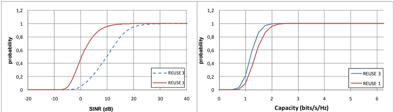
Figure 4 and 5: cdf of the SINR and the cell average throughput for fixed reuse schemes R1 and R3
