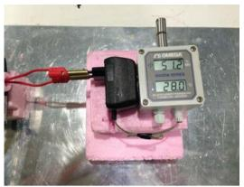
Fig 7. Electronic thermometer used as a susceptible EUT
