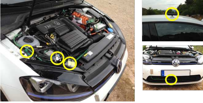
Fig. 5. Test vehicle instrumentation: Coolant flow meters and thermocouples in the motor compartment (left) and air thermocouples on the roof (top right) and in front of the cooler (bottom right).
