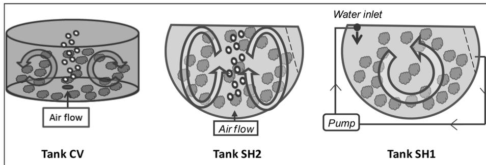
Figure 1: Tank configurations: CV(circular vertical aerated), SH2 and SH1(semicircular horizontal aerated and no aerated)
