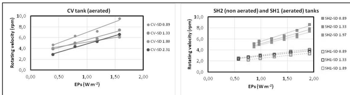
Figure 2: Rotational velocities obtained at different EPs in aerated tanks (CV and SH2) and no aerated tank (SH1).
