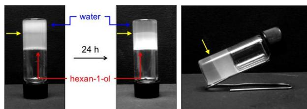
**Fig. 4** Phase-selective gelation and change in opacity of hexan-1-ol/water mixture after 24 h ( $c = 7 \text{ g L}^{-1}$ ). Total volume = 2 mL. Yellow arrow indicates the boundary between phases.
