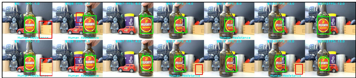
Figure 10: Detection results for a single object. Top Row: Detection output of the proposed method. Bottom Row: Output of the approach proposed in [52]. Green rectangles indicate object hypotheses whereas red ones are background hypotheses labeled by the user during the assistance.
