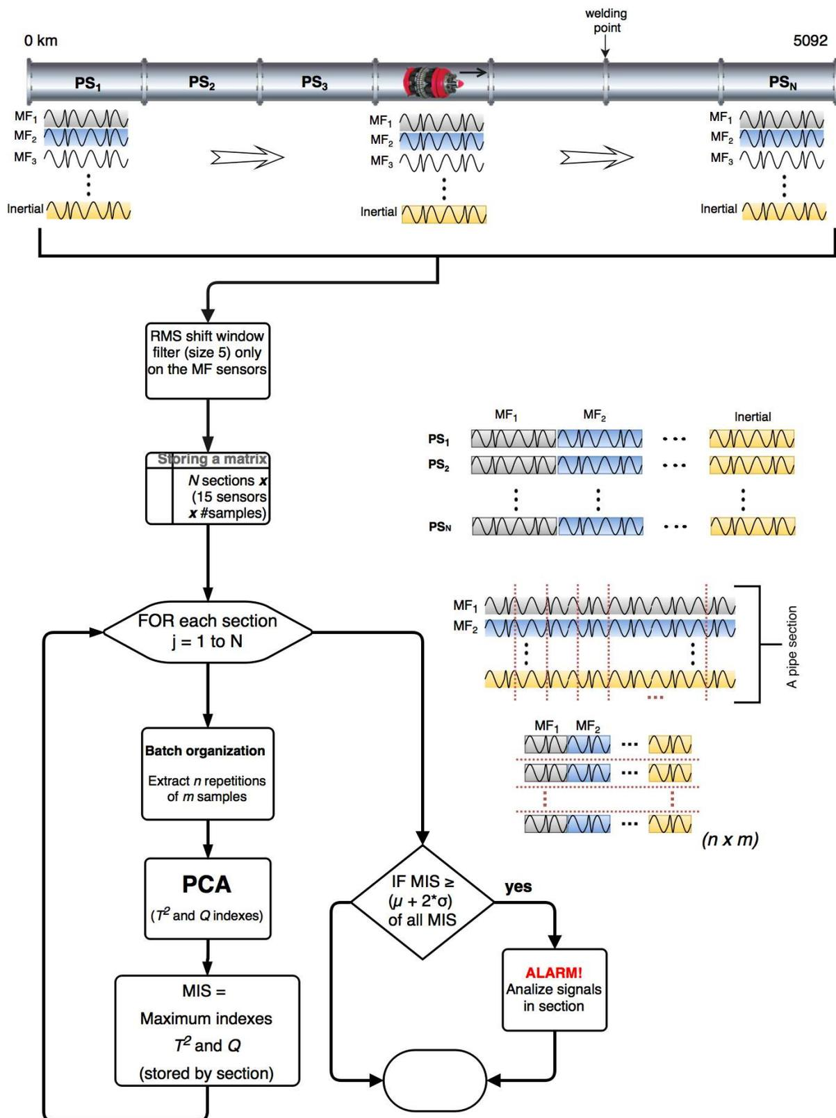
Figure 3: Methodological Steps followed to activate pipeline sections with potential changes
