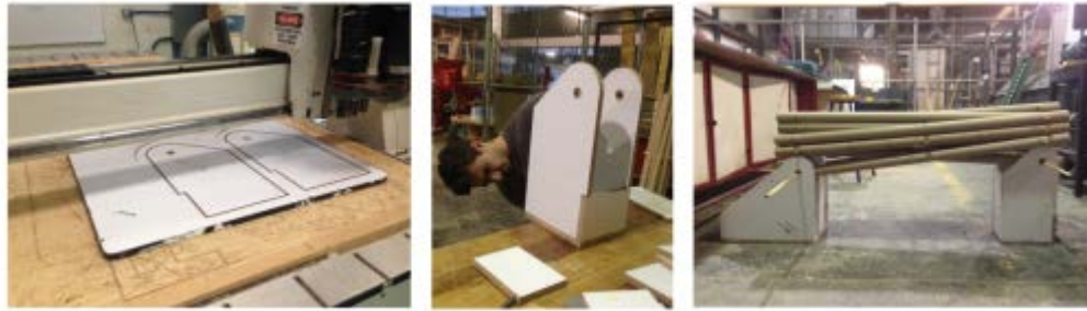
Figure 31. Base box construction.
