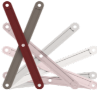
Figure 1. Scissor system where movement of the two articulated bars takes place at their center point.
