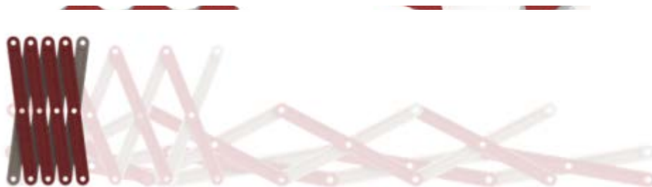
Figure 6. Scissor groups with a central pivot and linear deployment.
