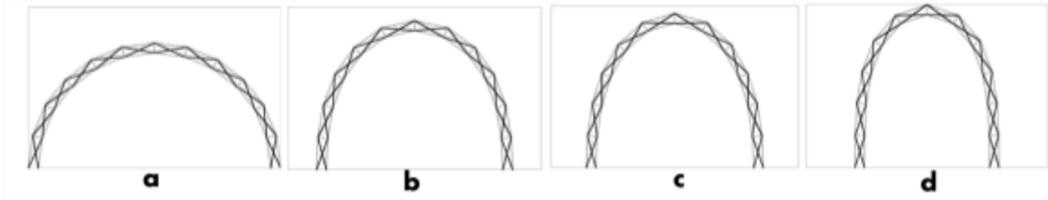
Figure 16. a) Equally dividing. b) Arithmetic progression. c) Geometric progression. d) Algebraic equation. (Babaei, 2009)
