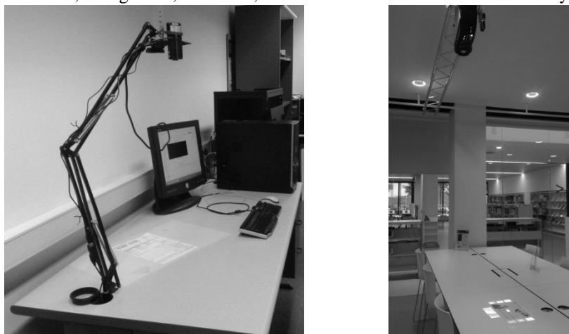
Figure 5. The initial setup of the nomadic system and fixed setup (right) built in a public library. The fixed setup has the projector/camera pair fixed in a structure that is attached to the ceiling. This way, the users have free space around them to experiment and freely perform gestures to interact with the application.
