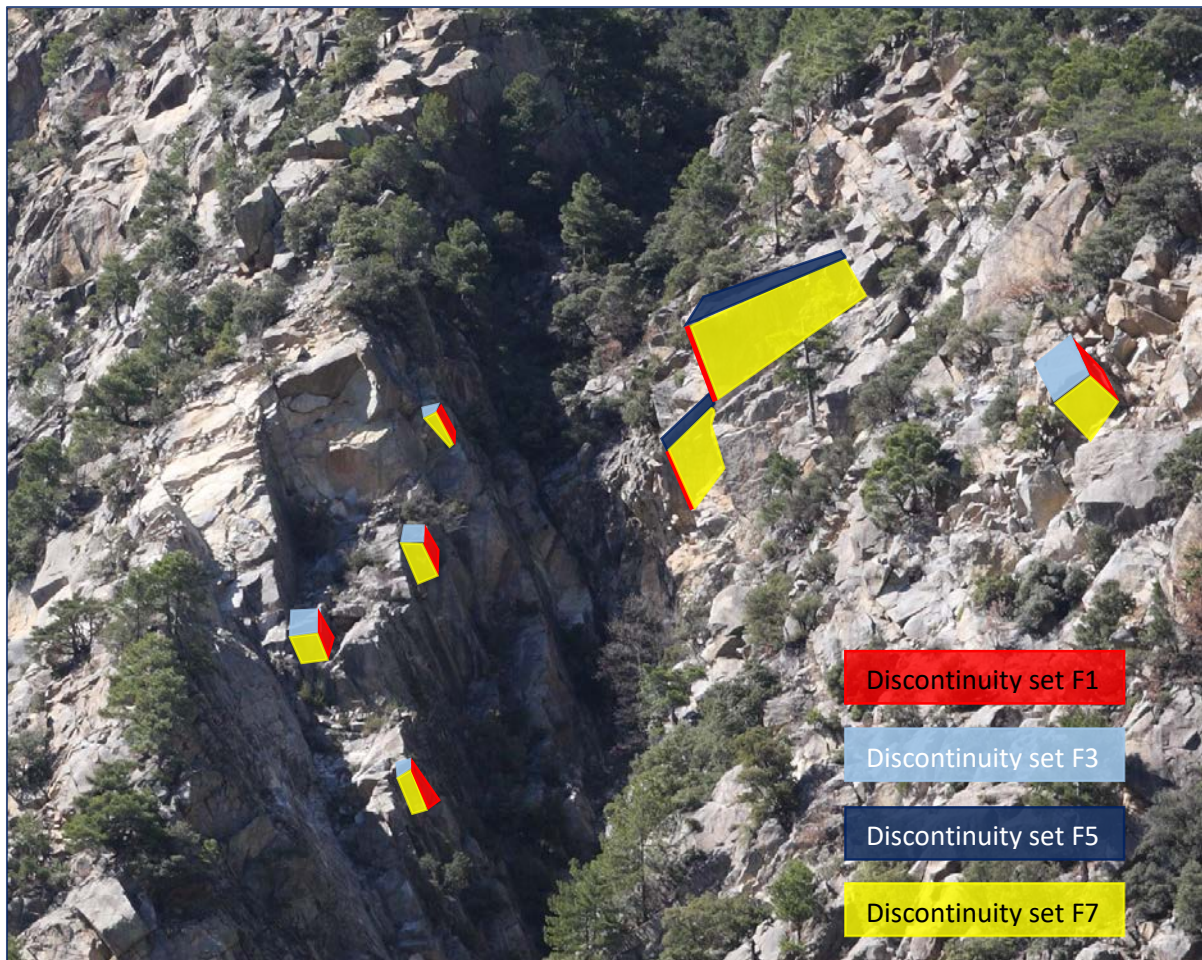
Fig. 4 Examples of intersection of discontinuity sets for the formation of rock blocks in the study-site
