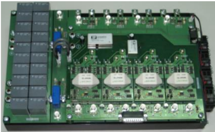
Fig. 6: Three-phase electronic power converter
