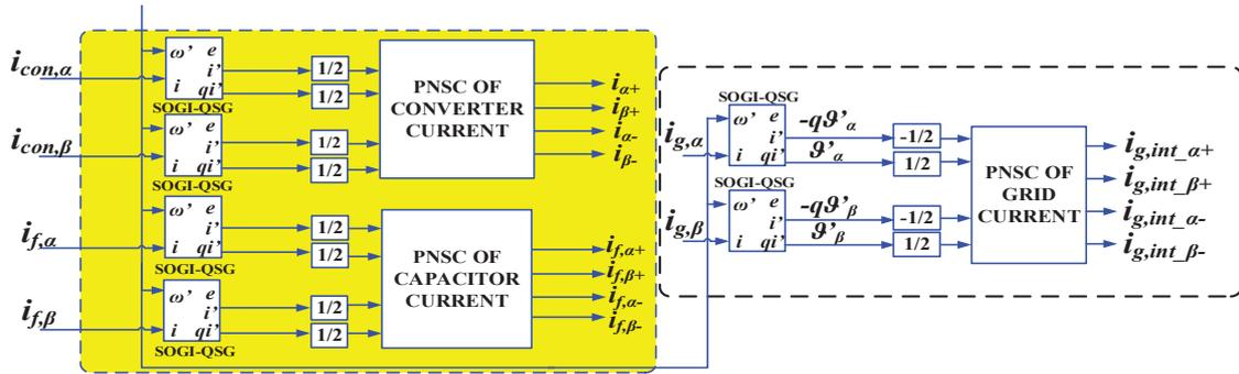
Fig. 4. Grid current integral and sequence separation of converter and capacitor current for Method 3
