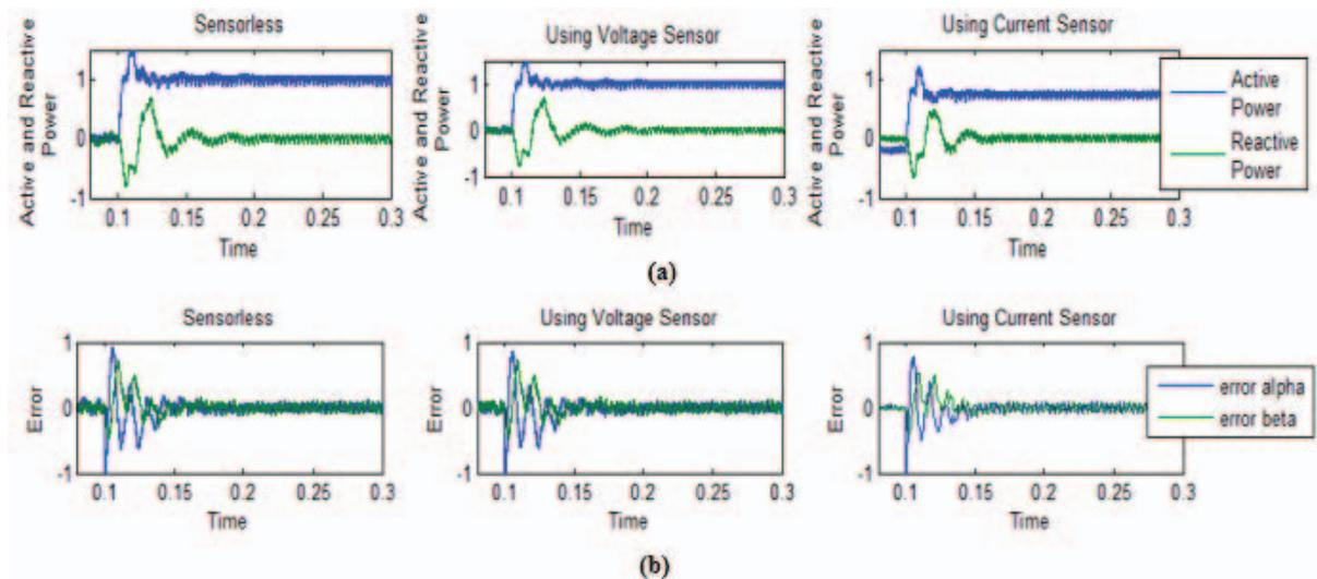
Fig. 6. Simulation results showing (a) Active and Reactive Power of the System, and (b) Steady State Error
