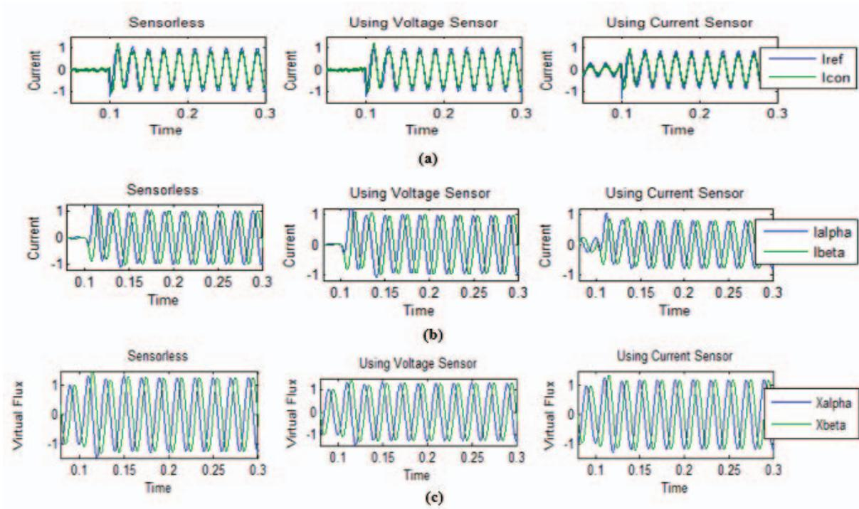
Fig. 5. Simulation Results (a) Reference Current and Converter Current. (b) Positive Sequence of Converter Current, and (c) Positive Sequence of Virtual Flux Estimation
