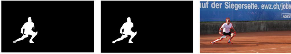
FIGURE 3.10: From left to right: particle stacking, represented by A_k^M , final state estimation x_k , represented by A_k^M > T_o , and overlay between the final estimated mask and the image I_k .
