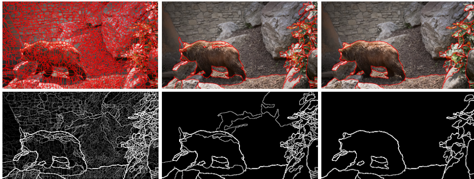
FIGURE 3.2: Different level of partition hierarchy. From left to right from the lowest hierarchy level \lambda = 0 to a higher one (rightmost) \lambda = 0.15 We can observe the amount of combinations (complexity) and the noise the lowest hierarchy offers and the segmentation errors at a higher (rightmost) one. The upper figures are the images with the partition overlay and the lower ones represent the segmentation hierarchy by means of the UCM map.
