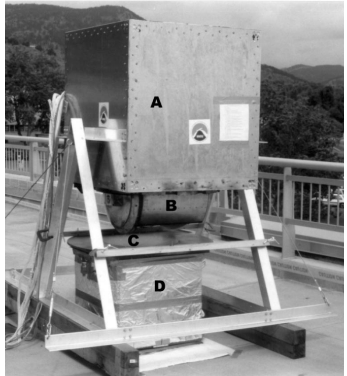
Fig. 2. NOAA fully polarimetric calibration experiment setup. (A) PSR housing, (B) PSR scanhead, (C) microwave retardation plate, and (D) linearly polarized standard.
